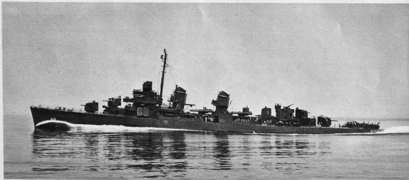
FLETCHERS' STACKS are broad, separated. Their lines are broken by searchlight platforms, control stations, in contrast to clean-stacked
